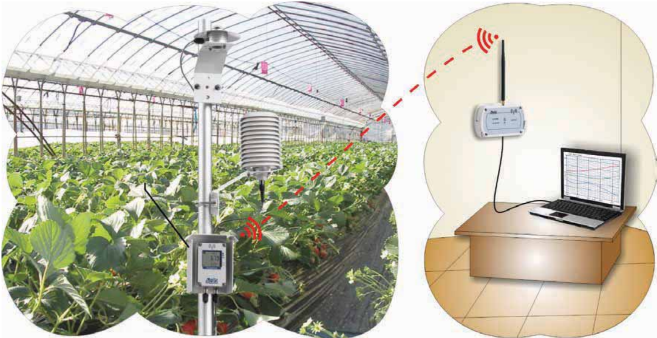
Outdoor transmitting station with data logger of the series HD35EDW...
