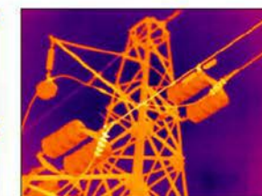
High voltage wire porcelain set overheating
