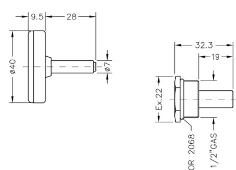
Bi-metal thermometer with rear stem, plastic casing and brass sheath; particularly suitable for under-floor heating systems.
