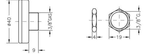
Bimetal thermometer with threaded rear stem and fixing nut, plastic casing and embossed glass; particularly suitable for refrigerating cells, display cabinets and cold counters.
