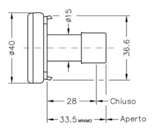
Bimetal Thermometer with specially shaped rear hooks for insertion on certain types of handles for ball valves. It allows the reading of the temperature of the liquid flowing in the pipeline intercepted by the ball valve.
