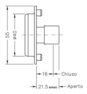
Bimetal Thermometer with specially shaped rear hooks for insertion on certain types of handles for ball valves. It allows the reading of the temperature of the liquid flowing in the pipeline intercepted by the ball valve.
