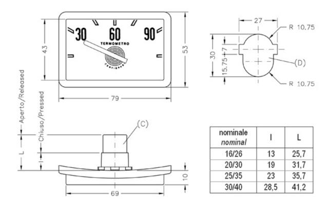
Bi-metal contact thermometer for water heater, with bayonet fixture.
